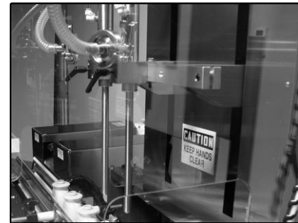
▲Positive shut-off nozzles prevent drips
